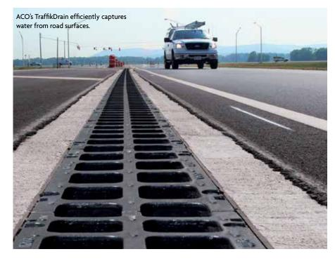
TraffikDrain and KerbDrain channels also require a shallower trench excavation compared to the kerb inlet pit and pipe system, which minimises the risk of interference with other services. Ease of maintenance is another advantage as trench drain blockage can be easier and quicker to remove in grated systems compared to underground pipe systems. In some cases, cleaning can take place without the grate needing to be removed.
